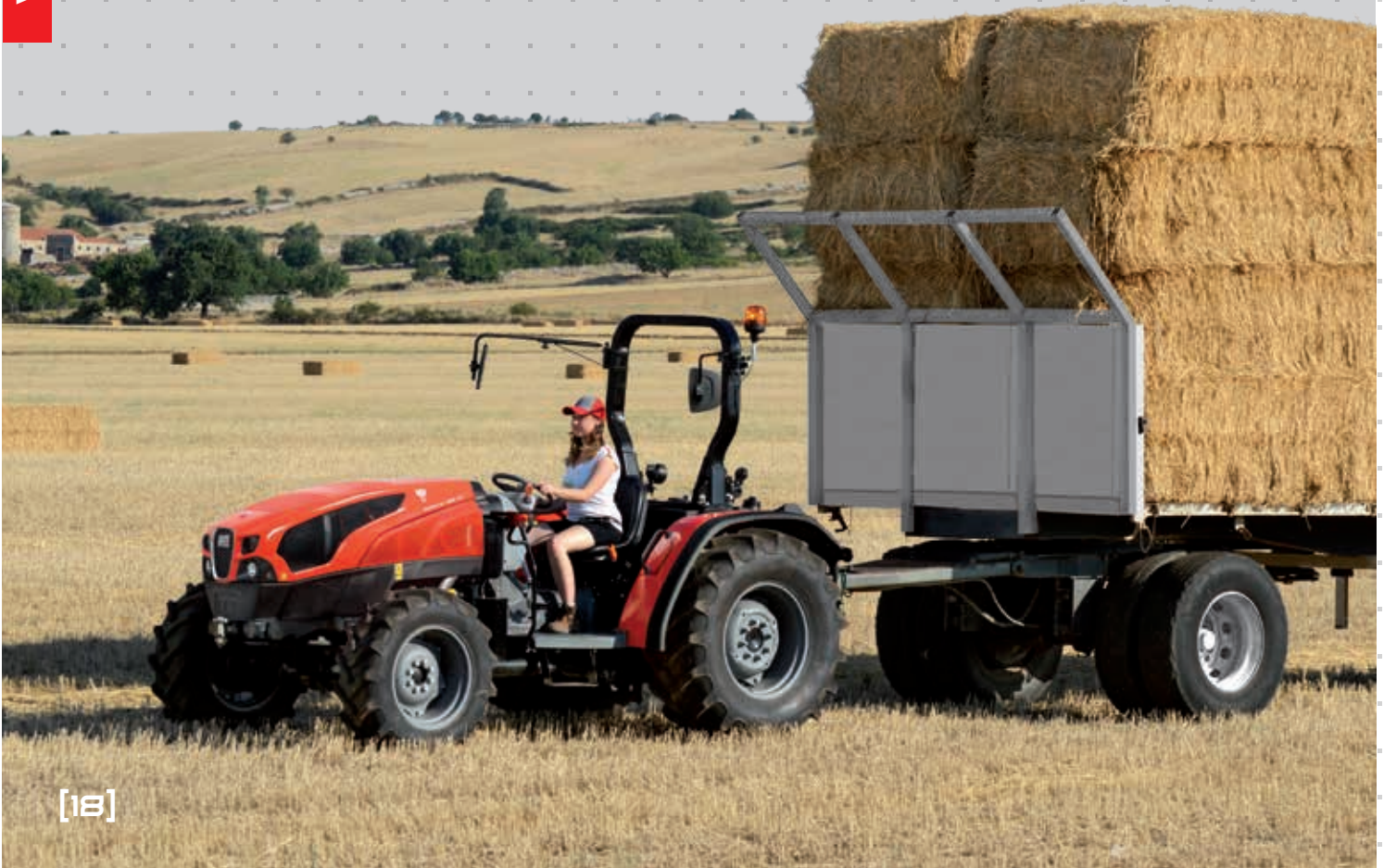
Hydraulic PowerShuttle with Stop&Go.
