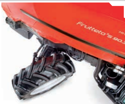
Superior manoeuvrability thanks to the high steering angle.
