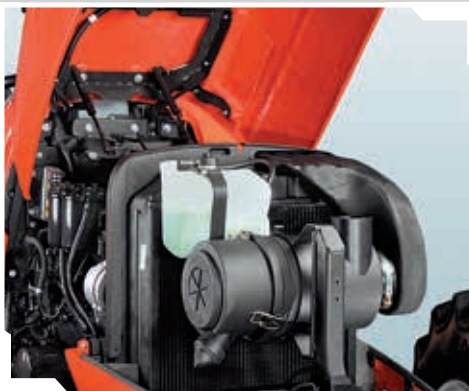
One piece fully tiltable bonnet.
