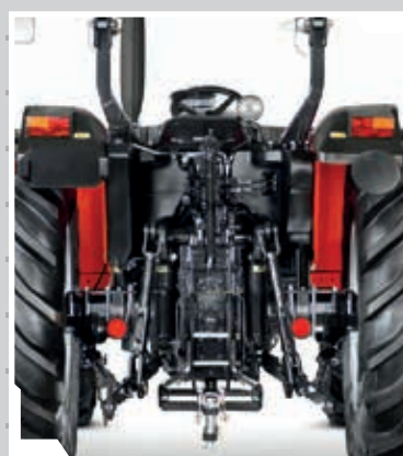
Rear lift capacity up to 4200 kg.
