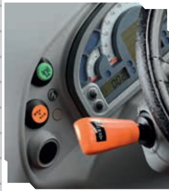
Hydraulic PowerShuttle with Stop&Go.
