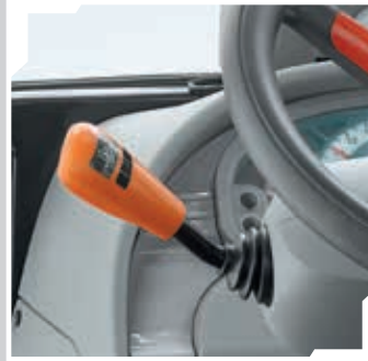
Hydraulic modulation for PowerShuttle sensitivity.
