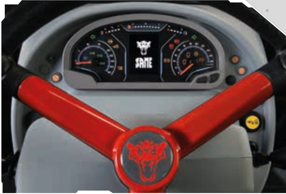
InfoCentre+ with a LCD display and two gauges
